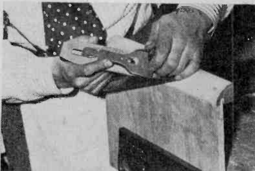
Fig. 5. Photo shows method used in shaping rounded corners of cabinet.
