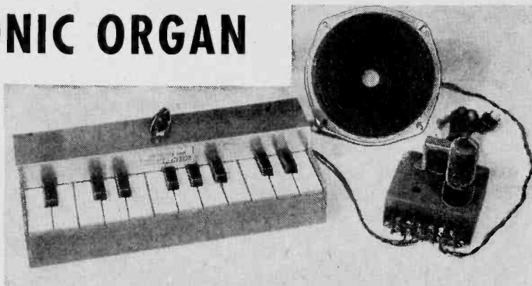
Completed electronic organ consists of: left, 20-key console with control providing 4 tone ranges; center, 5 in. PM speaker; and right, 1-tube oscillator.
