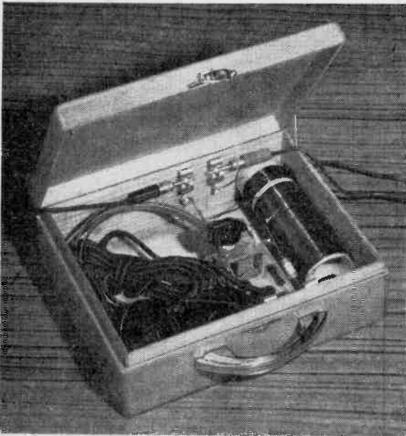
The crystal set is shown above mounted in the cigar box with headphones in place beside it.
