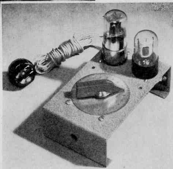
Flashlight beam focused on phototube at right can actuate the electronic control. Closeup of finished "eye" is shown at right.
