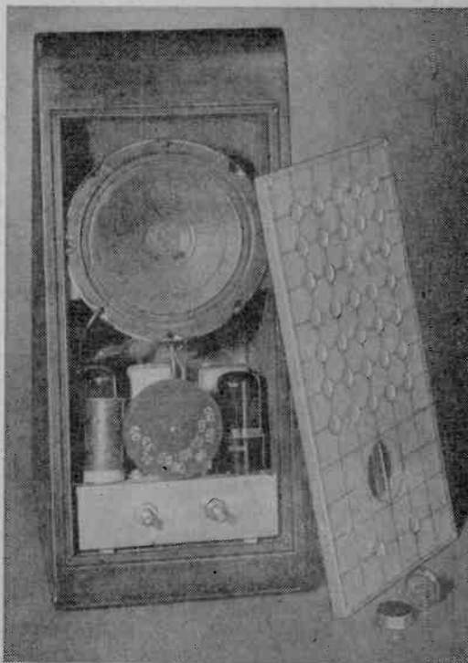
Cabinet with dial knobs and plastic panel removed, showing receiver and speaker units in place.
